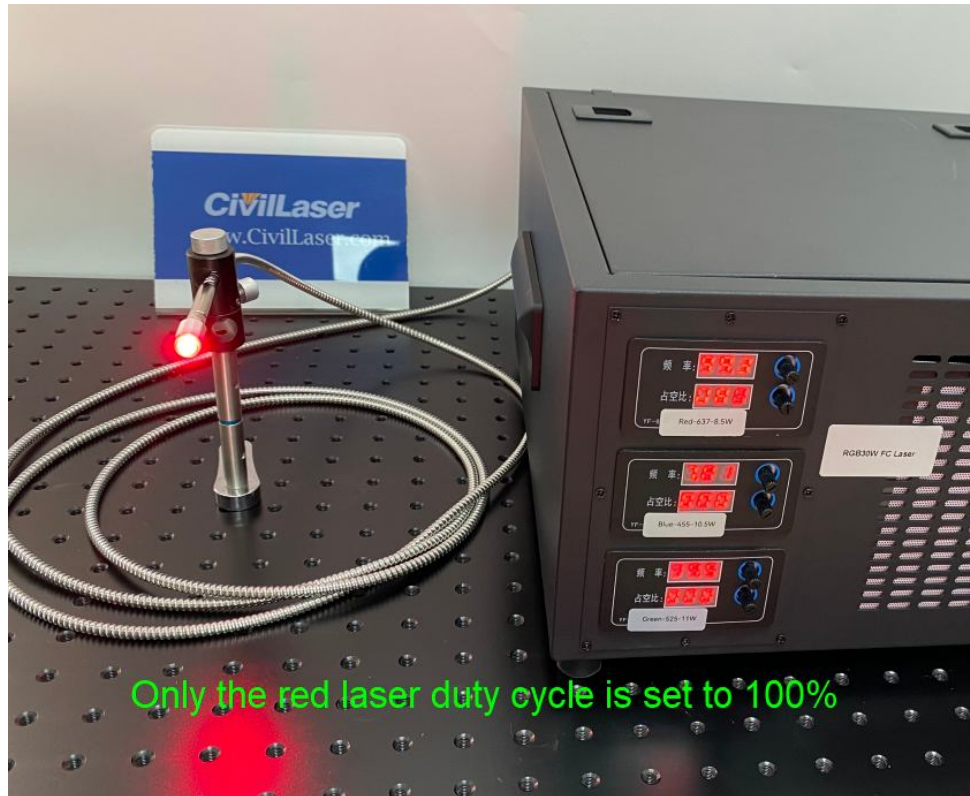
Only the red laser duty cycle is set to 100%
