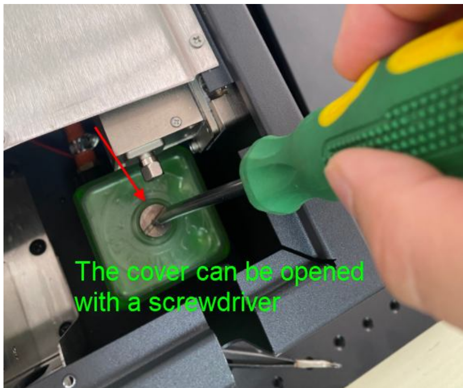
The cover can be opened with a screwdriver
